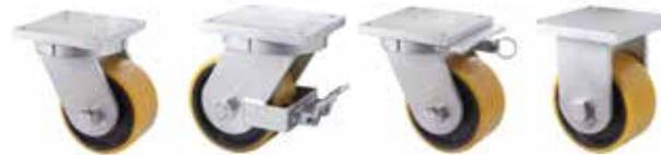
AZP Plate with swivel AZPBR Plate with swivel and wheel brake AZPDL Plate with swivel and direction lock AZF Fixed plate, no swivel
